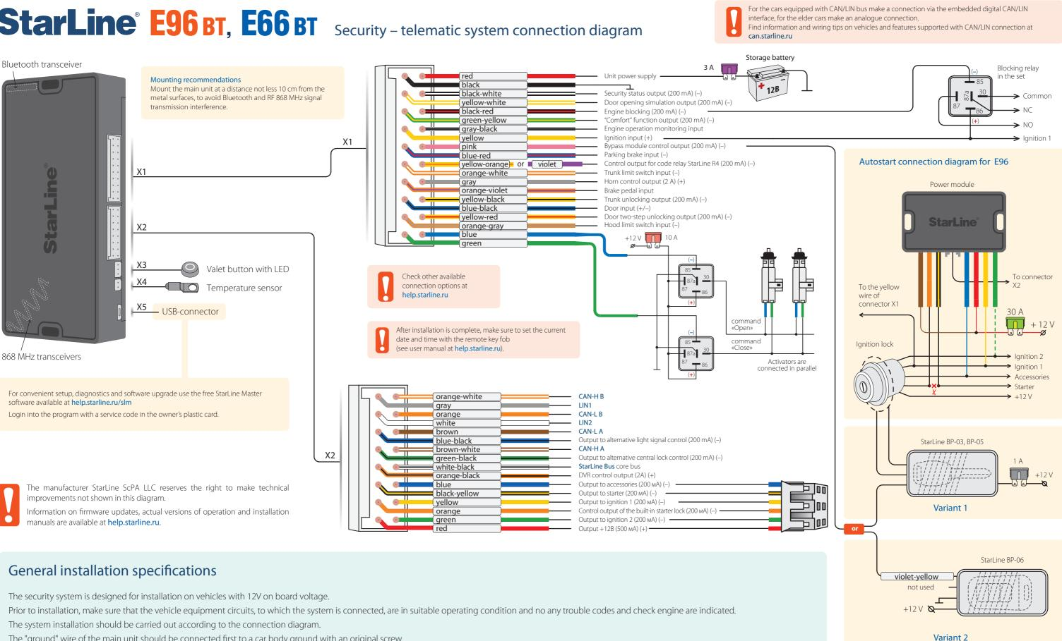
The "ground" wire of the main unit should be connected first to a car body ground with an original screw.
