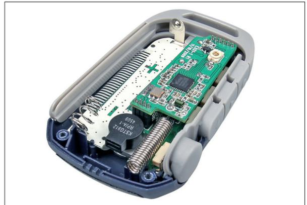
**Example of antenna built into the remote control unit**
