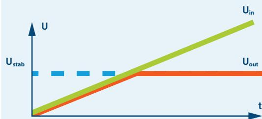
**Using a Zener diode for output voltage stabilization**
