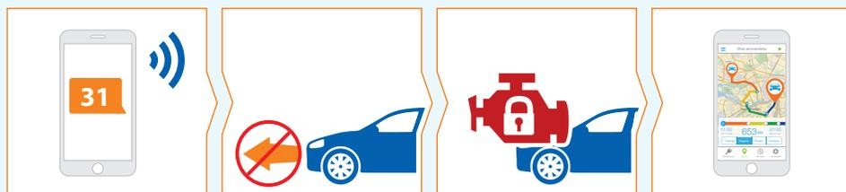
**Attention!** In case of a tag loss or battery discharge, SMS message will be sent to the phone and engine will be blocked when ignition is switched on. To continue a trip, put the tracker into Valet mode (SMS command 51). Remember that all security functions are disabled in the Valet mode!
